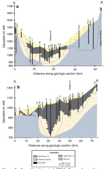
Figure 3 – From Hopkins et al. 2014. Figure shows the thickness of the confining layer in two different cross sections (referenced in Figure 1) across the Middle San Pedro basin. Notably the confining layer in general thins toward the upstream end (right hand side of bottom panel of figure).
