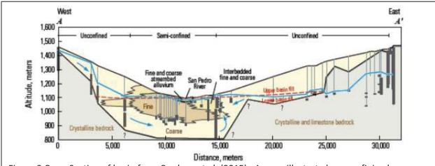
Figure 2 Cross Section of basin from Cordova et al. (2015). Arrows illustrate how confining layer can induce hydrologic discharges and effects distant form recharge and pumping locations.
