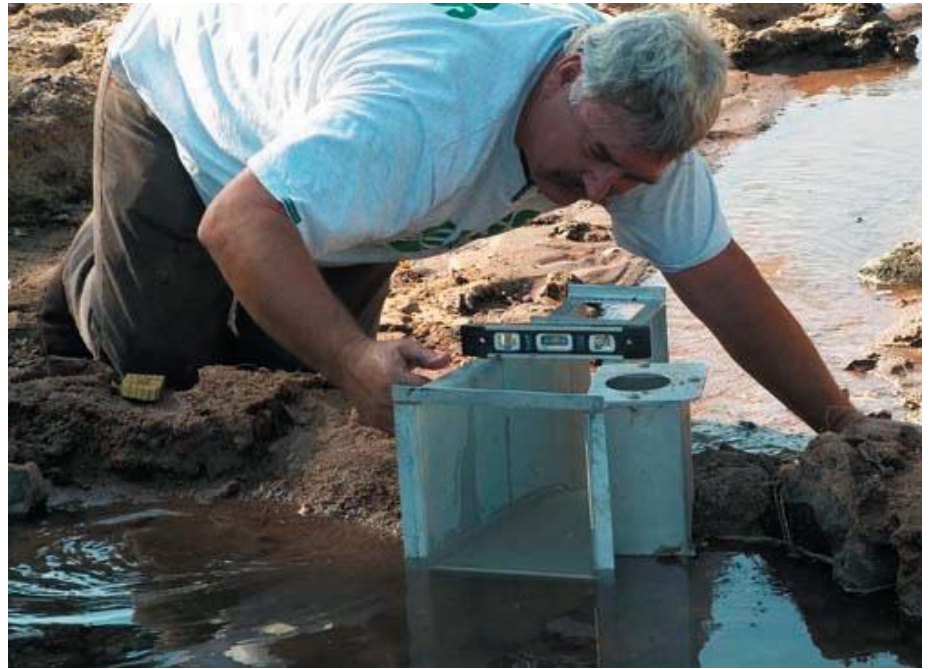
Emmet McGuire, a hydrologic technician with the U.S. Geological Survey, levels a portable flume earlier this week to check on the flow of the San Pedro River near the agency’s Charleston gauge. (Bill Hess-Herald/Review)
